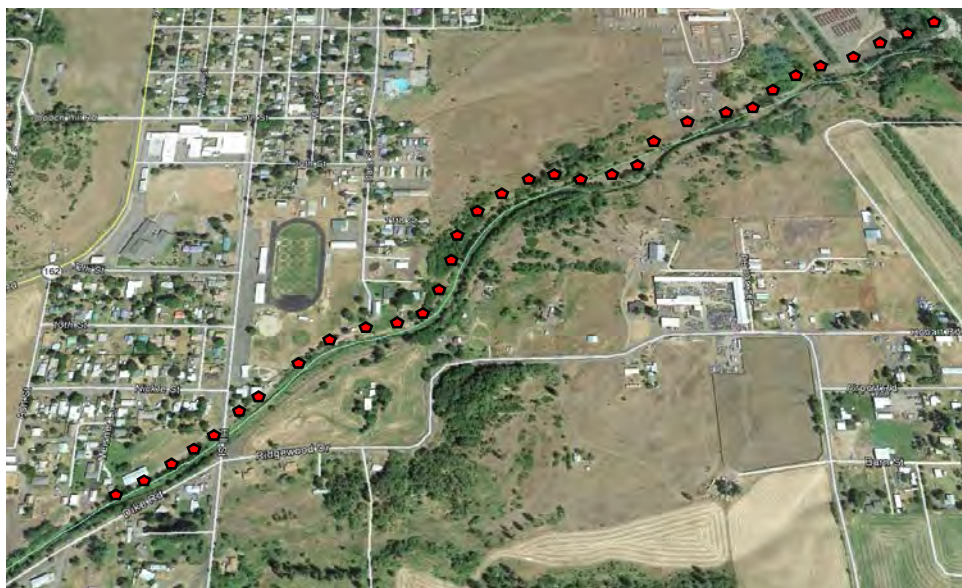
Figure 2. Potential temporary setback levee extents to protect the City of Kamiah, Idaho against increased flood potential.
